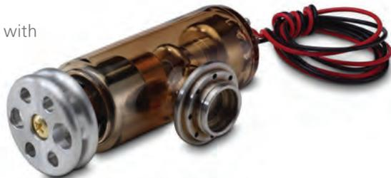
The 1550 Series X-ray tube can also be supplied in a stainless steel, lead-lined package that is filled with dielectric oil that enables the unit to provide maximum X-ray shielding and heat dissipation; this configuration is our popular Apogee 5500 Series packaged tube, which includes high voltage and filament connectors making it ideal for plug and play operation.
